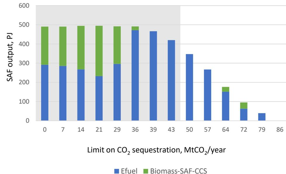
UK SAF production in 2050 (PJ yr<sup>-1</sup>), from net zero scenarios with varying degree of CCS constrained in the UK TIMES energy system model. Grey area cover scenarios that achieve net zero through imported emissions credit
