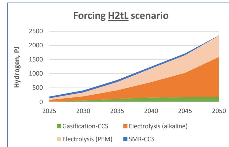
Hydrogen production methods for two scenarios designed to impose e-fuels in the energy system to meet 50% of UK's aviation demand in 2050 (~300 PJ)
