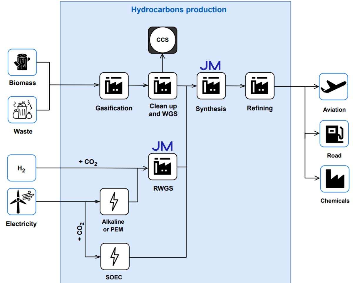
This diagram represents syngas pathways. Other opportunities that can convert biogenic resources into hydrocarbons are not reflected here (i.e. anaerobic digestion, fermentation, pyrolysis or hydrothermal liquefaction)
